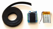
(a) A NodeMCU board and a small battery pack can easily be made wearable using VelcroWrap.
