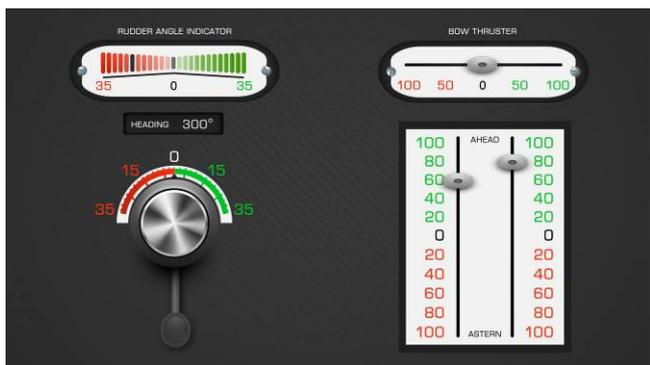
Figure 2. Example screen of Virtual Handles with rudder and machine telegraph.
