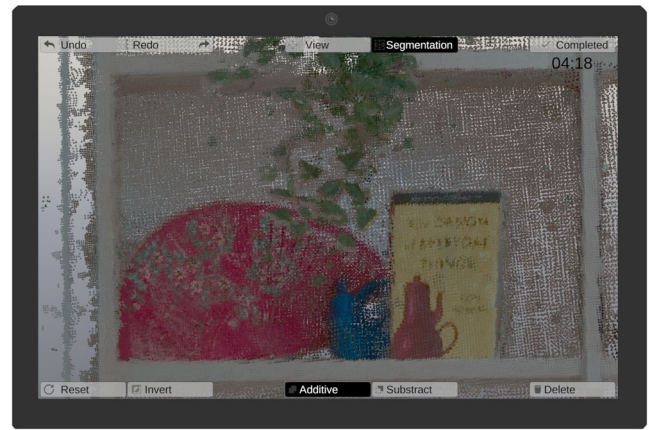
Figure 3. Interface of the tablet application. The buttons are grouped based on their semantic similarity, Undo ↶ and Redo ↷, View ↻ and Segmentation 🗒, Revert ↶ and Invert 🔄, Additive ➕ and Subtractive ➖, Delete 🗑, and Completed ✓. General functionalities are positioned at the top, and segmentation functionalities are at the bottom.
