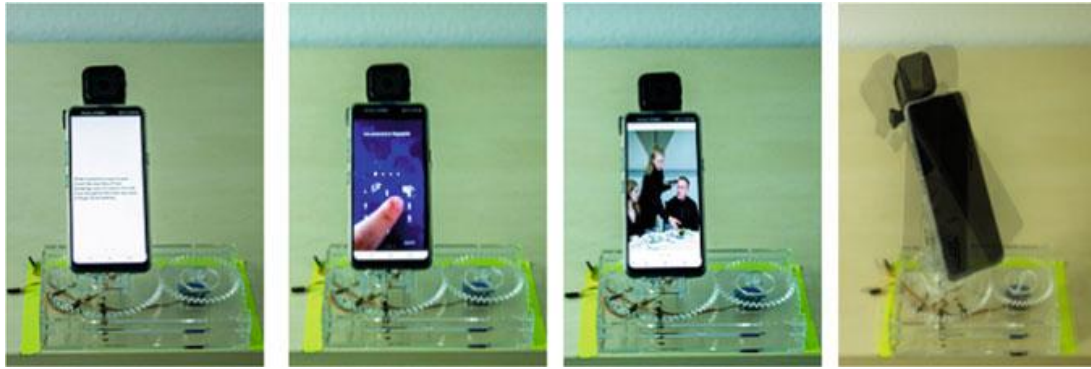
Fig. 4 Study apparatus to investigate the influence of distance and viewing angle on shoulder surfing success rate, figure taken from Bâce et al. [6] licensed under CC BY-NC-ND 4.0. The subfigures show examples of different content types on the phone display: (left to right): text, PIN, photo, and no content visible. The mechanical prototype visible rotated the smartphone between 0, 30, and 60°
