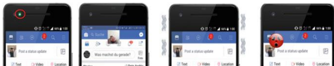
Fig. 5 Different feedback conditions to communicate a shoulder surfing incident investigated in previous work [44]. The different feedback conditions are (from left to right): (1) front LED, (2) video preview, (3) vibro-tactile, and (4) on-screen icon. The authors found that vibro-tactile feedback results in the lowest reaction time
